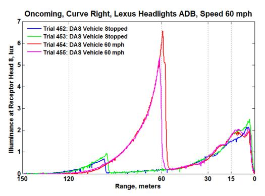
**Figure 20.** Illuminance Versus Distance for Lexus in ADB Mode Driving 60 mph (96.6 kph) in a Right Curved Roadway With DAS Vehicle Oncoming, Adjacent Lane at 0 or 60 mph (96.6 kph)
