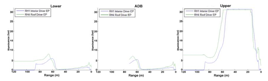
Figure 12. Illuminance Versus Distance by Headlighting System Mode - Dip Series (Straight) Oncoming, Adjacent Lane Maneuver, Small DAS 0 mph, Lexus
