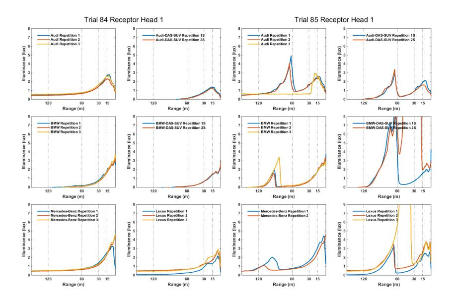
**Figure 86.** Lower Beam and ADB Illuminance Versus Distance for Oncoming, ADB Curves Right, Adjacent Lane, DAS 62 mph, ADB 62 mph, Trial 84 (Lower Beam) and Trial 85 (ADB)
