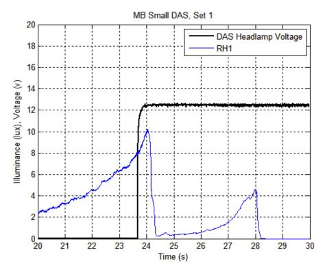
**Figure 53.** Graph of ADB Adaptation Response to Suddenly Appearing DAS Vehicle Headlighting System, Small DAS Vehicle, Mercedes-Benz
