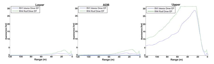
**Figure 7.** Illuminance Versus Distance by Headlighting System Mode - Straight, Oncoming, Adjacent Lane Maneuver, Small DAS, BMW
