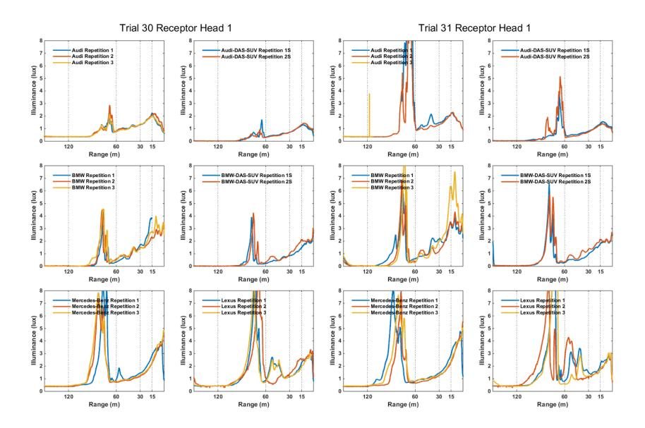
Figure 82. Lower Beam and ADB Illuminance Versus Distance for Oncoming, Winding, DAS 0 mph, ADB 62 mph, Trial 30 (Lower Beam) and Trial 31 (ADB)
