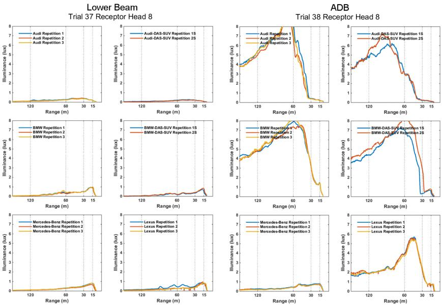
**Figure 64.** Lower Beam and ADB Illuminance Versus Distance for Oncoming 90° Intersection Maneuver Scenario With DAS Vehicle 0 mph, ADB Vehicle 62 mph (99.8 kph)
