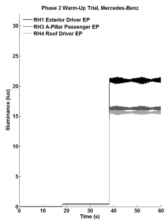
**Figure 47.** Mercedes-Benz Warm-Up Trial Example Showing Ambient Illumination, Lower Beam, Upper Beam Modes for Small DAS Vehicle, Phase 2
