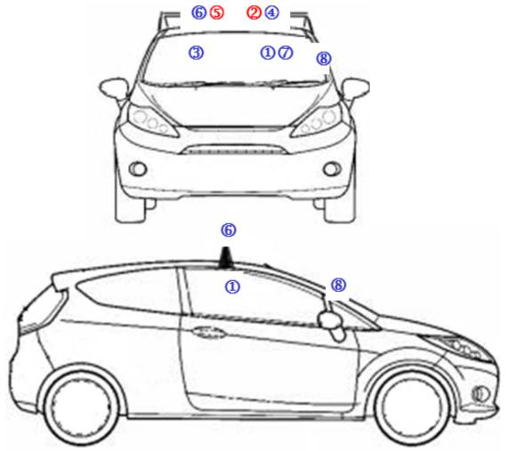
Figure 3. Illuminance Measurement, Receptor Head Positioning on DAS Vehicle, Phase 1
