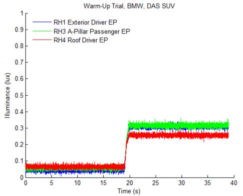
**Figure 44.** BMW Warm-Up Trial Example Showing Ambient Illumination, Lower Beam Mode for SUV DAS Vehicle, Phase 2
