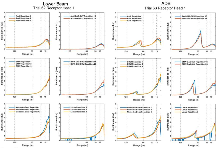
**Figure 66.** Lower Beam and ADB Illuminance Versus Distance for Oncoming Curve Left Scenario With DAS and ADB Vehicles Driving 62 mph (99.8 kph)
