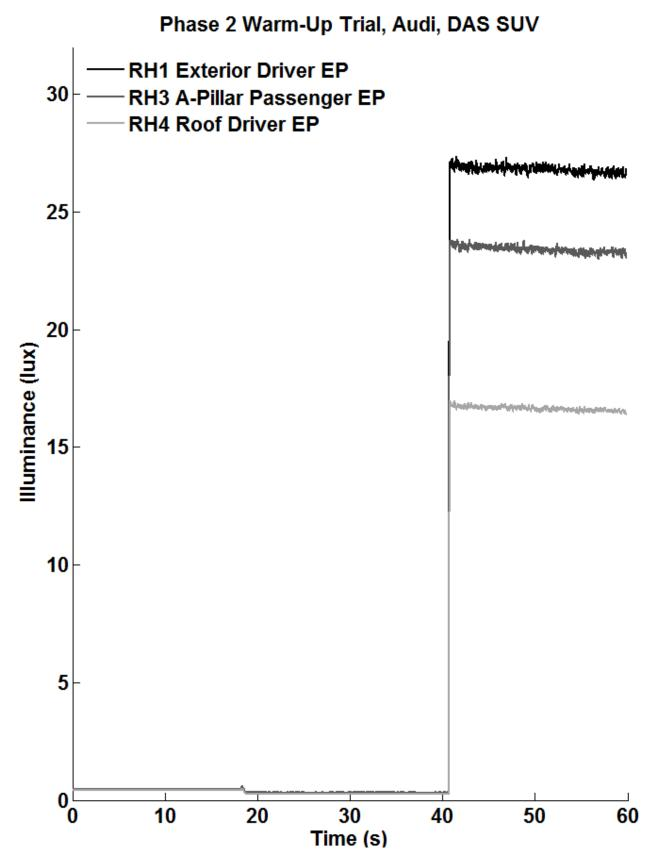
**Figure 38.** Audi Warm-Up Trial Example Showing DRL, Lower Beam, Upper Beam Modes for SUV DAS Vehicle, Phase 2
