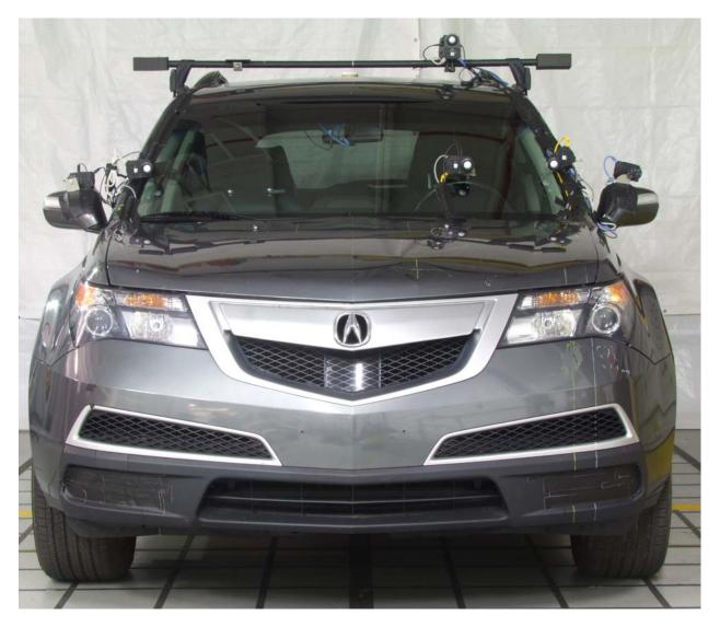
Figure 27. SUV DAS (Acura MDX) Front
