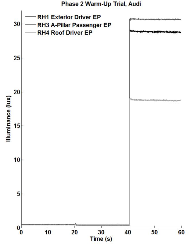
**Figure 37.** Audi Warm-Up Trial Example Showing DRL, Lower Beam, Upper Beam Modes for Small DAS Vehicle, Phase 2
