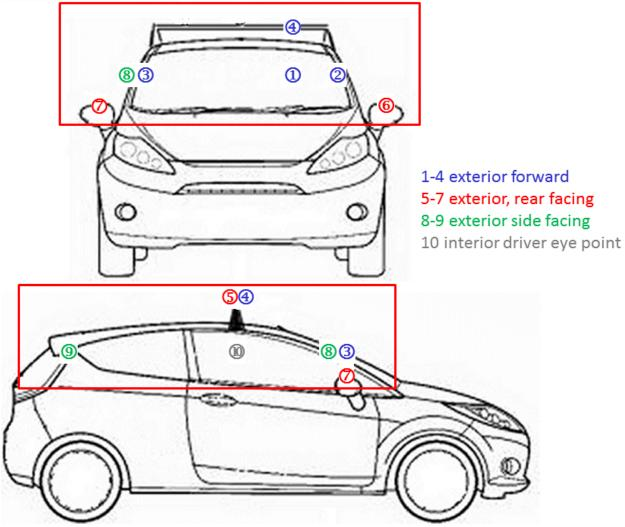
Figure 76. Possible Objective Test Illuminance Measurement Regions
