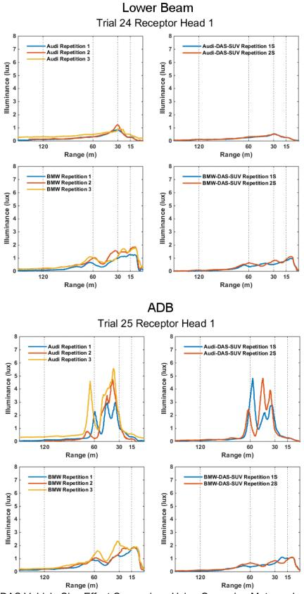
**Figure 72.** DAS Vehicle Size Effect Comparison Using Oncoming Motorcycle Scenario (Both vehicles traveling 62 mph; 99.8 kph)
