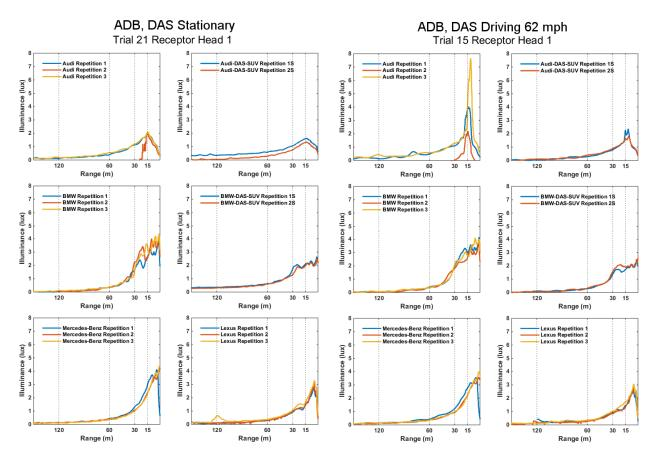
**Figure 73.** ADB Illuminance Versus Distance in Oncoming, Straight Maneuver Scenario for DAS Vehicle Stationary Versus Driving 62 mph (99.8 kph)
