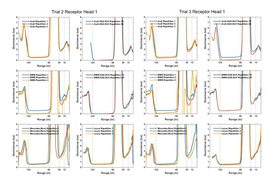
**Figure 77.** Lower Beam and ADB Illuminance Versus Distance for Oncoming, Straight, Dip, Adjacent Lane, DAS 0 mph, ADB 62 mph, Trial 2 (Lower Beam) and Trial 3 (ADB)
