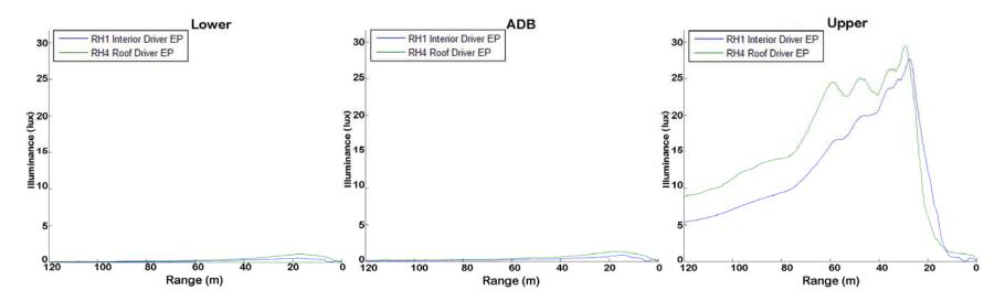
Figure 6. Illuminance Versus Distance by Headlighting System Mode - Straight, Oncoming, Adjacent Lane Maneuver, Small DAS, Audi
