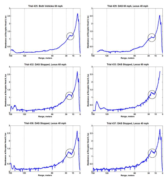
**Figure 21.** Example of Noteworthy ADB Headlighting System Behavior Documented in Trials With the Lexus Test Vehicle
