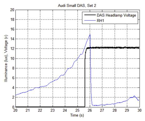
**Figure 50.** Graph of ADB Adaptation Response to Suddenly Appearing DAS Vehicle Headlighting System, Small DAS Vehicle, Audi
