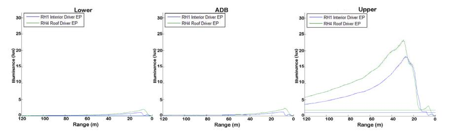
Figure 9. Illuminance Versus Distance by Headlighting System Mode - Straight, Oncoming, Adjacent Lane Maneuver, Small DAS, Mercedes-Benz
