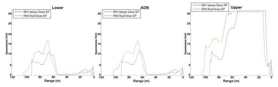
Figure 11. Illuminance Versus Distance by Headlighting System Mode - Dip Series (Straight) Oncoming, Adjacent Lane Maneuver, Small DAS 0 mph, BMW
