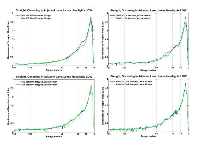
**Figure 18.** Illuminance Versus Distance as a Function of ADB and DAS Vehicle Speeds for Oncoming, Straight, Adjacent Lane Maneuver, Lower Beam Mode, Lexus
