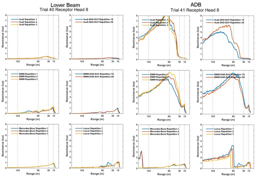
**Figure 65.** Lower Beam and ADB Illuminance Versus Distance for Oncoming 60° Intersection Maneuver Scenario With DAS Vehicle 0 mph, ADB Vehicle 62 mph (99.8 kph)
