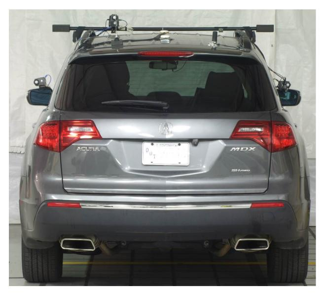
Figure 28. SUV DAS (Acura MDX) Rear
