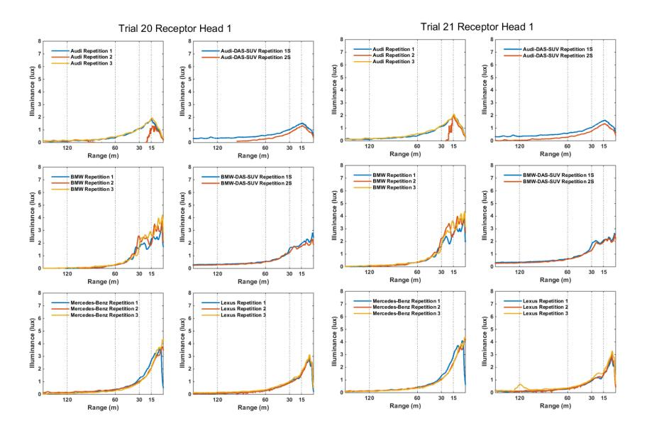
**Figure 79.** Lower Beam and ADB Illuminance Versus Distance for Oncoming, Straight, Adjacent Lane, DAS 0 mph, ADB 62 mph, Trial 20 (Lower Beam) and Trial 21 (ADB)
