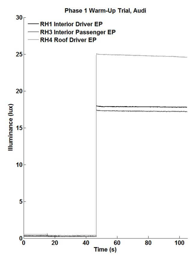
**Figure 4.** Example Warm-Up Trial, Audi A8 (Vertical Order of Channels Shown in Upper Beam Portion of Graph, From Top to Bottom, is RH4, RH1, RH3)
