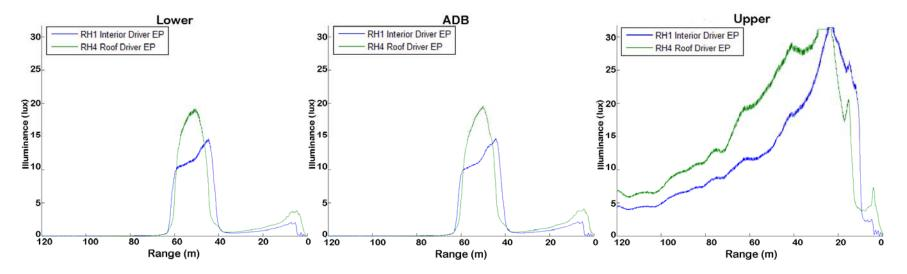
Figure 13. Illuminance Versus Distance by Headlighting System Mode - Dip Series (Straight) Oncoming, Adjacent Lane Maneuver, Small DAS 0 mph, Mercedes-Benz
