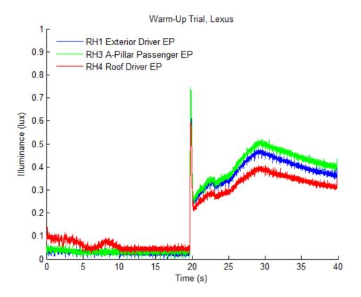
**Figure 46.** Lexus Warm-Up Trial Example Showing Ambient Illumination, Lower Beam Mode for Small DAS Vehicle, Phase 2
