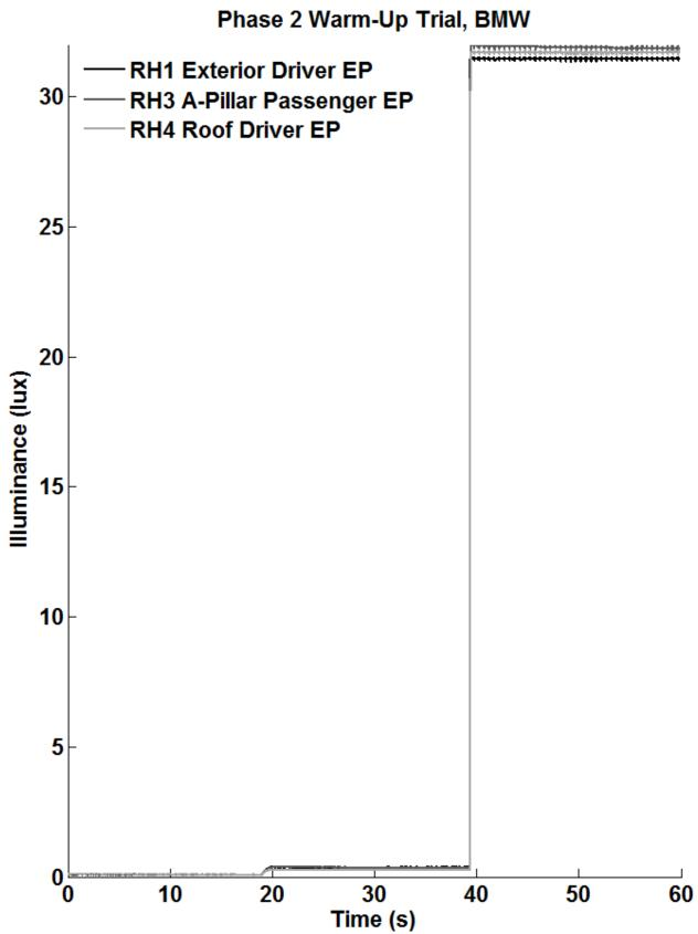
**Figure 41.** BMW Warm-Up Trial Example Showing DRL, Lower Beam, Upper Beam Modes for Small DAS Vehicle, Phase 2
