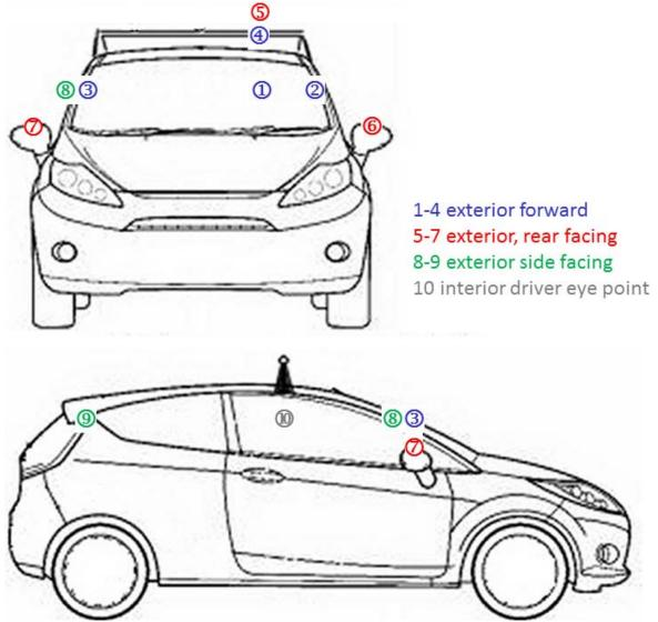
Figure 31. Illuminance Measurement Receptor Head Positioning on DAS Vehicle, Phase 2
