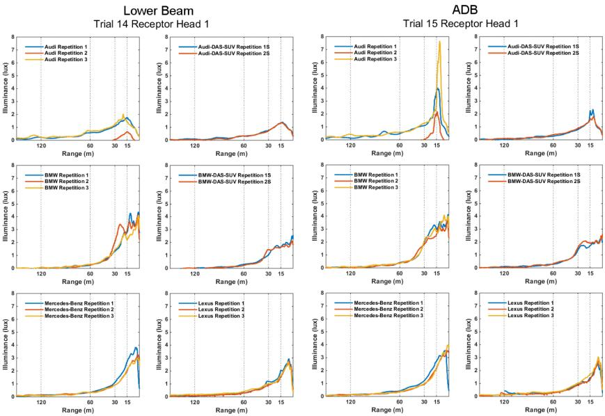
**Figure 61.** Lower Beam and ADB Illuminance Versus Distance for Oncoming Straight Maneuver Scenario With DAS Vehicle Driving 62 mph (99.8 kph)
