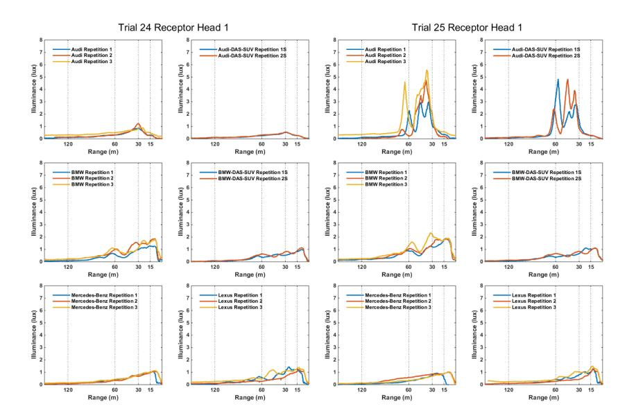
**Figure 81.** Lower Beam and ADB Illuminance Versus Distance for Oncoming, Straight, Motorcycle, Adjacent Lane, DAS 62 mph, ADB 62 mph, Trial 24 (Lower Beam) and Trial 25 (ADB)
