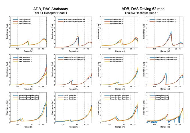
**Figure 74.** ADB Illuminance Versus Distance in Oncoming, Left Curve Maneuver Scenario for DAS Vehicle Stationary Versus Driving 62 mph (99.8 kph)
