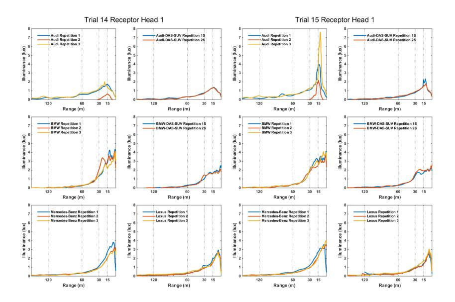
**Figure 78.** Lower Beam and ADB Illuminance Versus Distance for Oncoming, Straight, Adjacent Lane, DAS 62 mph, ADB 62 mph, Trial 14 (Lower Beam) and Trial 15 (ADB)
