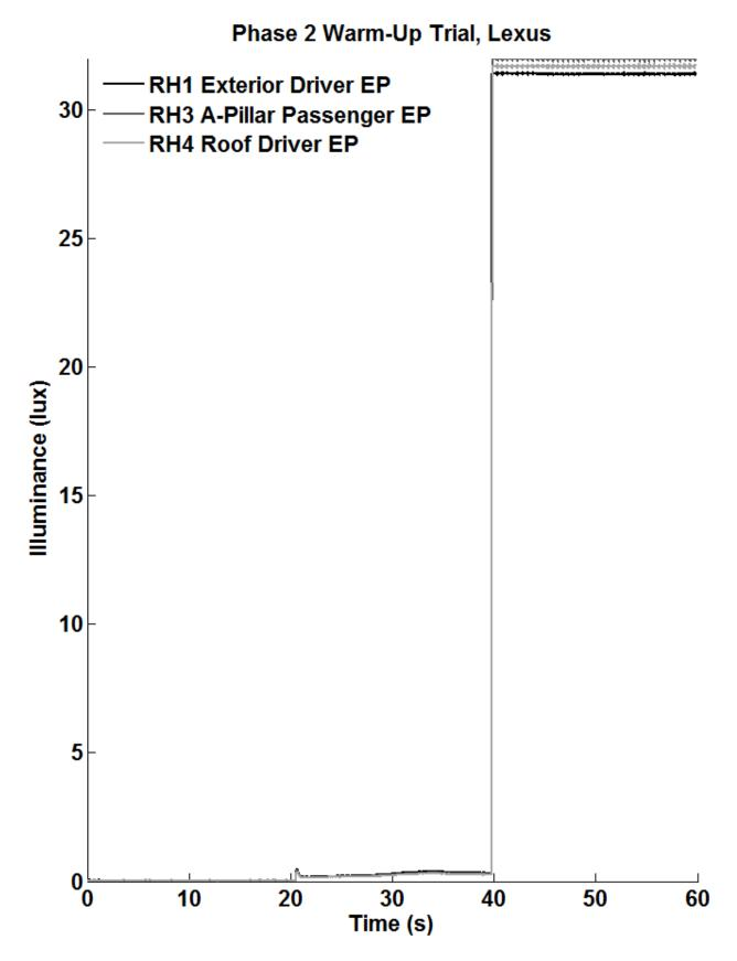
**Figure 45.** Lexus Warm-Up Trial Example Showing Ambient Illumination, Lower Beam, Upper Beam Modes for Small DAS Vehicle, Phase 2
