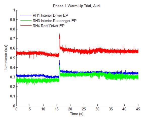
**Figure 5.** Example Warm-Up Trial First 45 Seconds, Audi A8 (Vertical Order of Graphed Channels From Top to Bottom is RH4, RH1, RH3)
