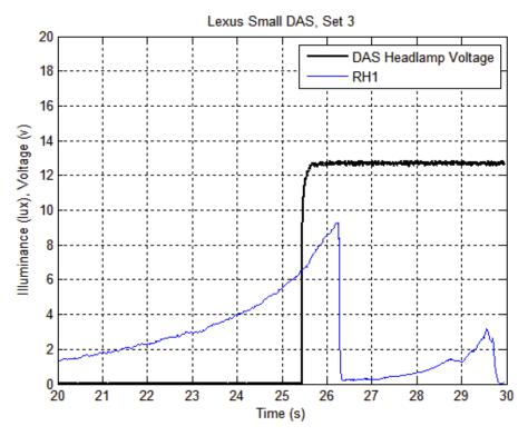
**Figure 52.** Graph of ADB Adaptation Response to Suddenly Appearing DAS Vehicle Headlighting System, Small DAS Vehicle, Lexus
