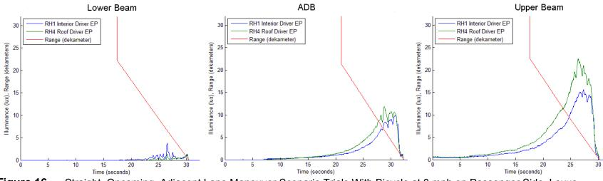
Figure 16. Straight, Oncoming, Adjacent Lane Maneuver Scenario Trials With Bicycle at 0 mph on Passenger Side, Lexus
