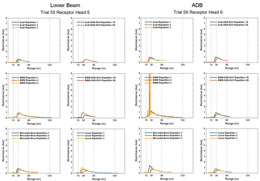
**Figure 70.** Lower Beam and ADB Illuminance Versus Distance for Same-Direction Curve Left Passive Passing (DAS Vehicle at 62 mph (99.8 kph) Passes ADB Vehicle at 45 mph (72.4 kph)) Scenario
