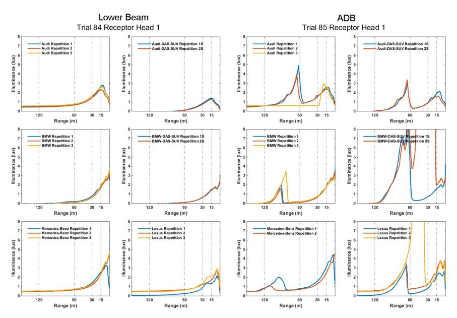
**Figure 67.** Lower Beam and ADB Illuminance Versus Distance for Oncoming Curve Right Scenario With DAS and ADB Vehicles Driving 62 mph (99.8 kph)
