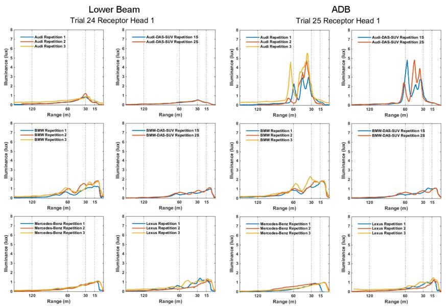
**Figure 62.** Lower Beam and ADB Illuminance Versus Distance for Oncoming Straight Maneuver Scenario With Motorcycle Driving 62 mph (99.8 kph)
