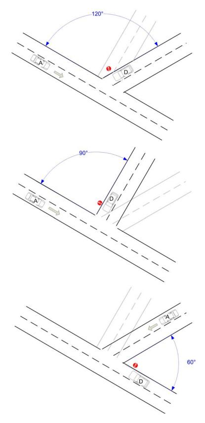
**Figure 23.** Intersection Scenarios: 60, 90, and 120-Degree Angled Approaches (A=ADB vehicle at 62 mph (96.6 kph); D = DAS vehicle at 0 mph)
