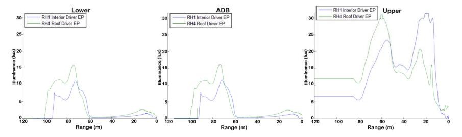
Figure 10. Illuminance Versus Distance by Headlighting System Mode - Dip Series (Straight) Oncoming, Adjacent Lane Maneuver, Small DAS 0 mph, Audi
