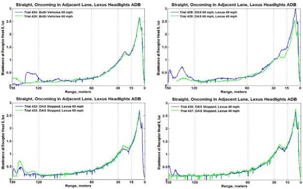
**Figure 19.** Illuminance Versus Distance as a Function of ADB and DAS Vehicle Speeds for Oncoming, Straight, Adjacent Lane Maneuver, ADB Mode, Lexus
