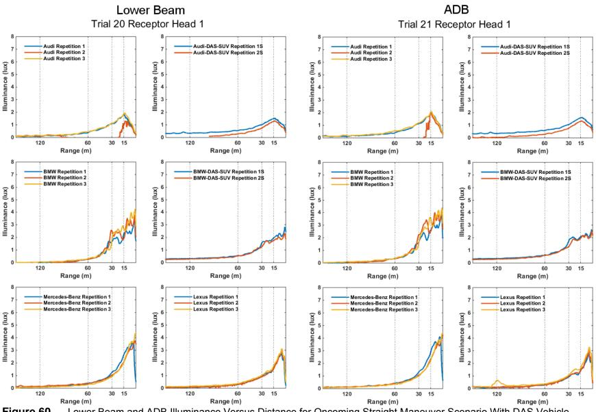
Figure 60. Lower Beam and ADB Illuminance Versus Distance for Oncoming Straight Maneuver Scenario With DAS Vehicle Stationary
