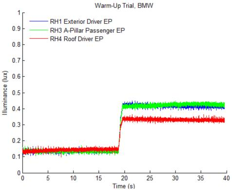
**Figure 43.** BMW Warm-Up Trial Example Showing Ambient Illumination, Lower Beam, Mode for Small DAS Vehicle, Phase 2
