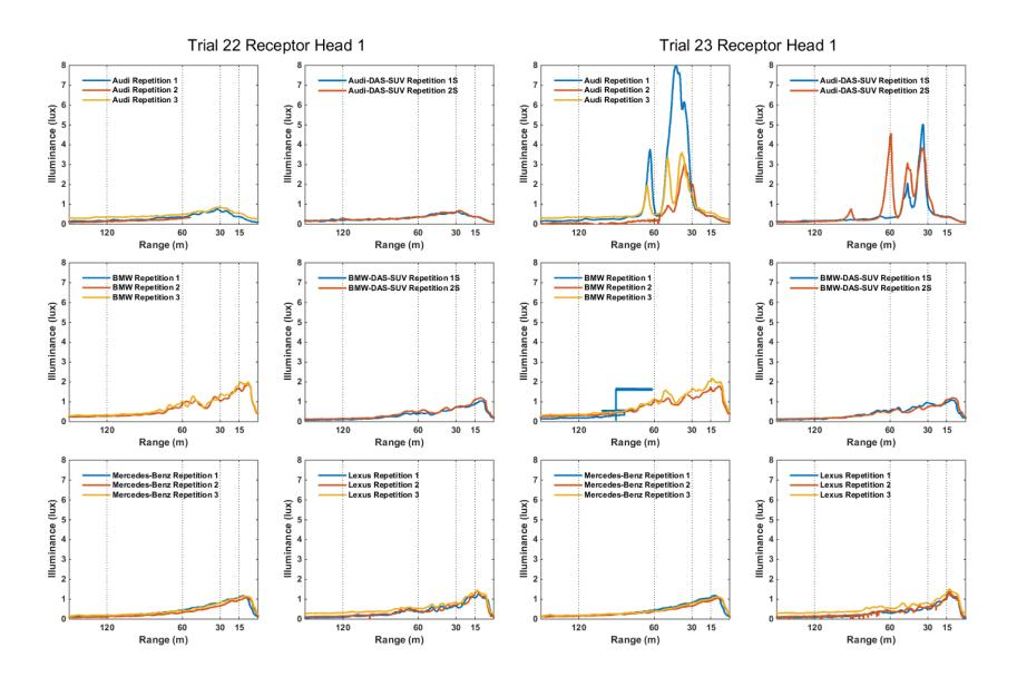
**Figure 80.** Lower Beam and ADB Illuminance Versus Distance for Oncoming, Straight, Motorcycle, Adjacent Lane, DAS 0 mph, ADB 62 mph, Trial 22 (Lower Beam) and Trial 23 (ADB) NOTE: NO VALID RANGE DATA for BMW Repetition 1 (Small DAS) for Trial 22 and only for range > 80 m for Trial 23
