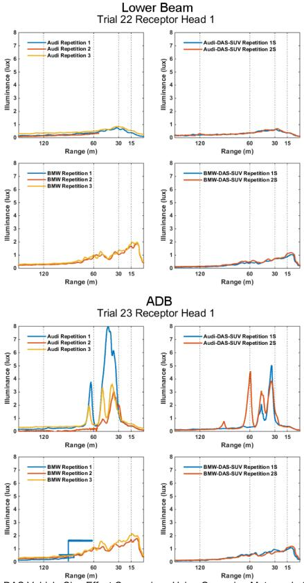
**Figure 71.** DAS Vehicle Size Effect Comparison Using Oncoming Motorcycle Scenario (DAS/Motorcycle 0 mph, ADB 62 mph (99.8 kph))
