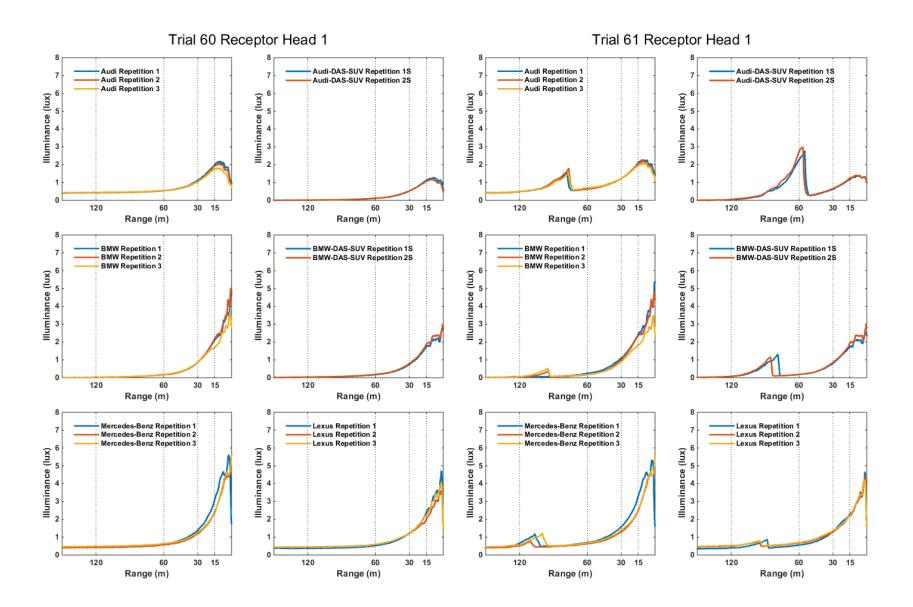
**Figure 83.** Lower Beam and ADB Illuminance Versus Distance for Oncoming, ADB Curves Left, Adjacent Lane, DAS 0 mph, ADB 62 mph, Trial 60 (Lower Beam) and Trial 61 (ADB)
