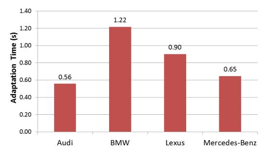
**Figure 49.** Average ADB Adaptation Time for Response to Suddenly Appearing DAS Vehicle Headlighting System
