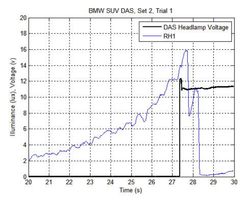
Figure 51. Graph of ADB Adaptation Response to Suddenly Appearing DAS Vehicle Headlighting System Illuminance, SUV DAS Vehicle, BMW
